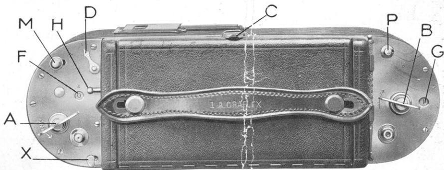
To decrease speed of shutter, release tension of spring by pushing escapement **P**, back and forth, until the required lower tension number is registered at **G**.
